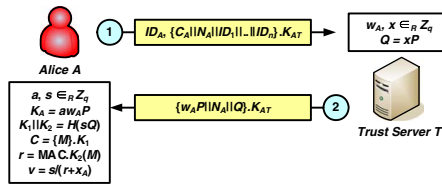
Fig. 4. The Sub-protocol between the Sender and the Server for Multiple Recipients
